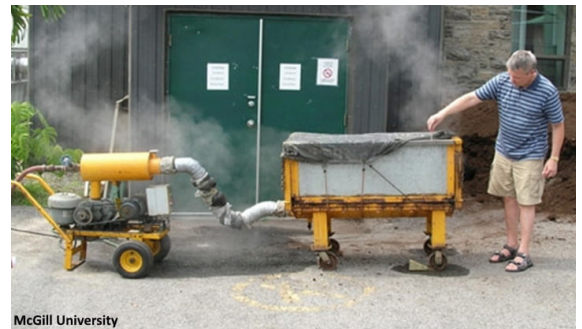
A steam pasteurizer that is used for soils can also be used to disinfect stakes. Photo: McGill University
